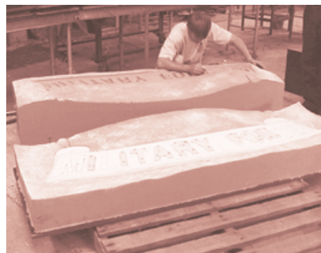
▲ Detailing a section of the mould after extraction of the pattern.
